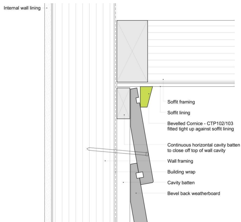
Bevel Back - Top Of Wall - Flat Soffit
